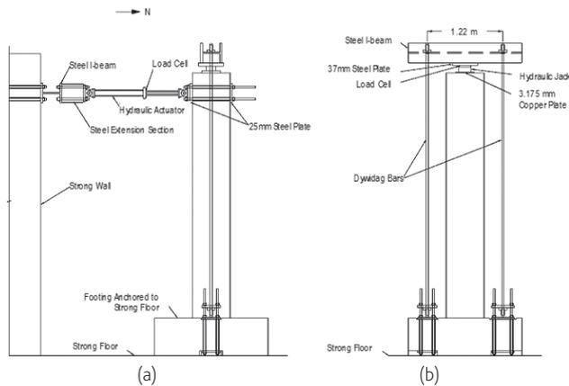
**Figure 2** Experimental setup: (a) lateral loading system; (b) axial force loading system
