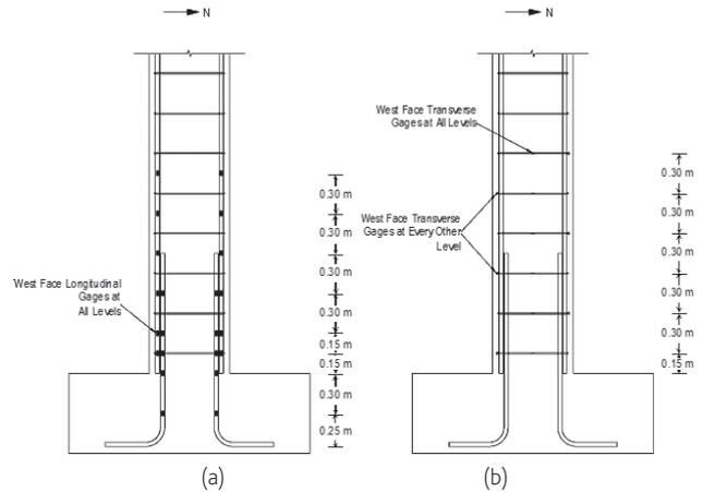
**Figure 3** Strain gage locations: (a) vertical reinforcing steel bars and (b) transverse reinforcing steel ties
