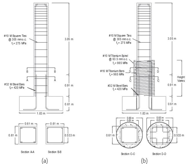
**Figure 1** Overall elevation view and cross sections of column specimens, including geometry and reinforcing details: (a) Specimen C1 = as-built configuration and (b) Specimens C2 and C3 = retrofitted configurations
