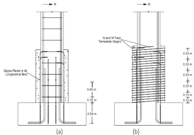
**Figure 4** Strain gage locations: (a) vertical TiABs and (b) spiral TiAB
