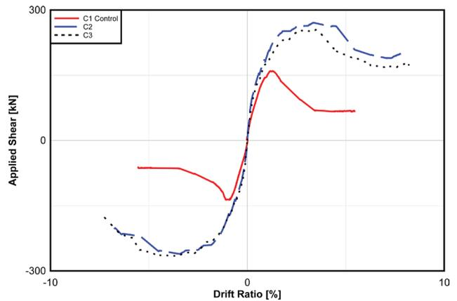
Figure 9 Backbone shear-drift responses for all specimens
