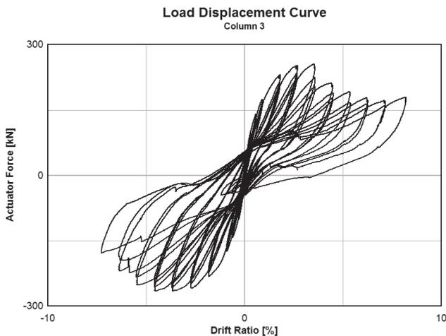
Figure 8 Overall lateral force-column top displacement response for specimen C3
