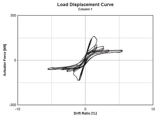
**Figure 6** Overall lateral force-column top displacement response for specimen C1
