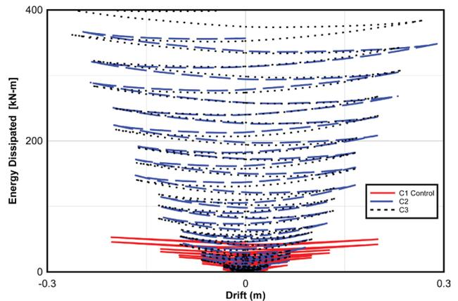
Figure 10 Energy dissipated at drift amplitude for all specimens
