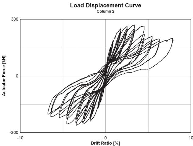
Figure 7 Overall lateral force-column top displacement response for specimen C2
