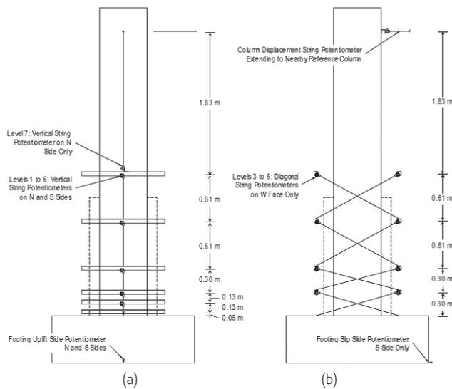
**Figure 5** External instrumentation setup for: (a) vertical deformations and (b) horizontal deformations
