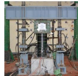
**Figure 4** Cyclic tests on 1:6 pier specimens (P1, P3, R1, R3): displacements histories applied on the pier specimens during cyclic tests; cyclic test setup at Fuzhou University Lab
