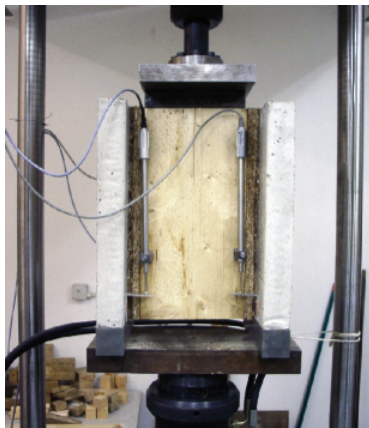
Figure 4 Push-out specimen for investigation of the structural behavior of shear connectors
