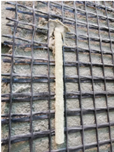
Figure 3 Specimen R2-OOP: Detail of the L-shape connector
