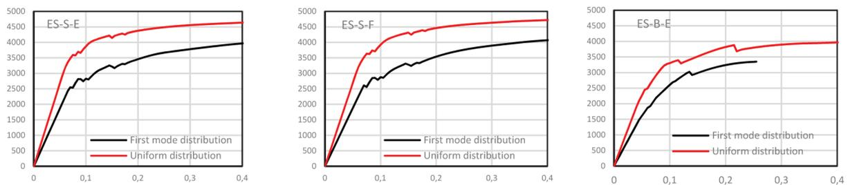
b) Pushover results for the refined models (Base Shear in kN, Top displacement in m)
