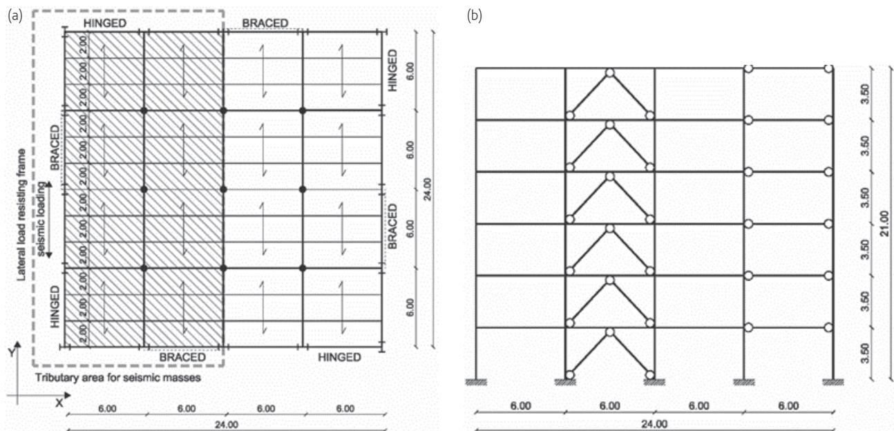
Figure 1 (a) Plan view and tributary area, (b) Elevation view of the perimeter frame
