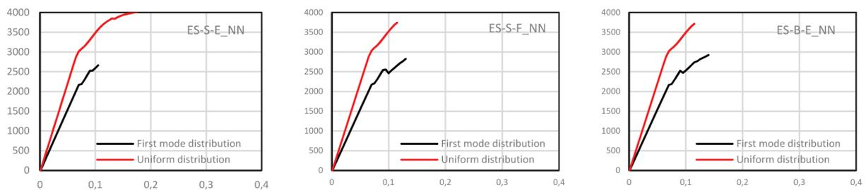
a) Pushover results for the simplified models (Base Shear in kN, Top displacement in m)
