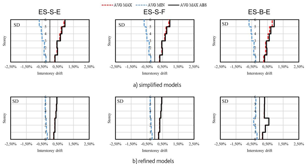
Figure 9 IDA – interstorey drift ratio at severe damage limit state
