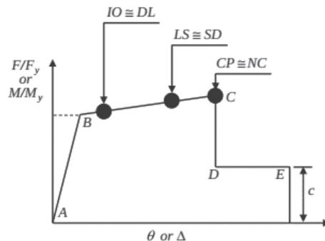
**Figure 2** Generalized acceptance criteria – damage state conditions [14]
