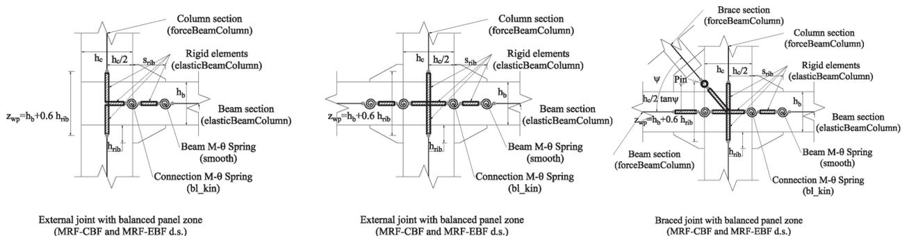
Figure 5 Rigid element models for joints with strong web panels (ES-S-E and ES-S-F)
