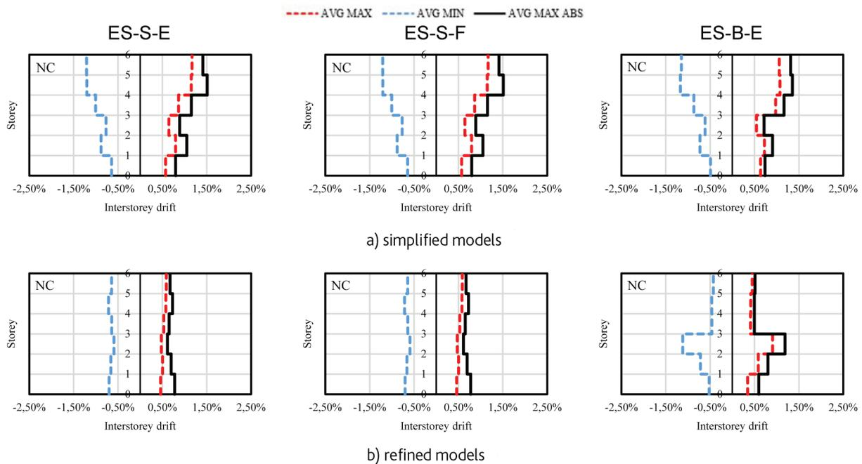
Figure 10 IDA – interstorey drift ratio at near collapse limit state
