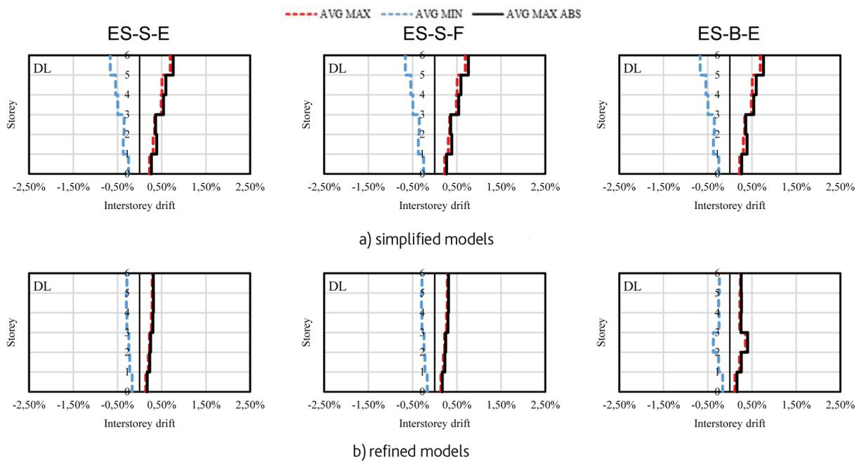
Figure 8 IDA – interstorey drift ratio at damage limitation limit state
