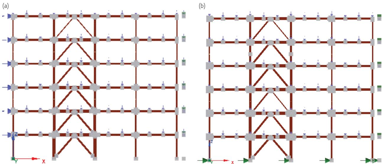
Figure 4 Loading for (a) pushover and (b) IDA
