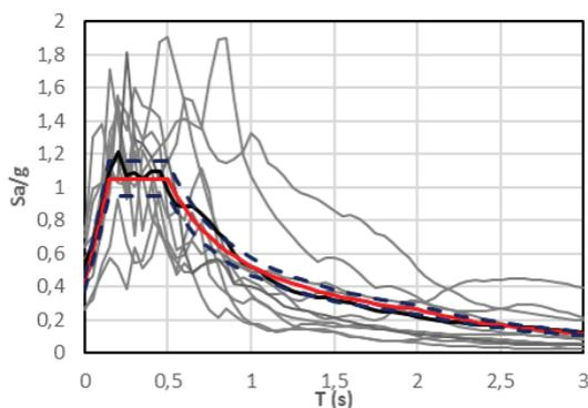
**Figure 3** EC8 response spectrum compared to the avg. spectrum of the ground motion records
