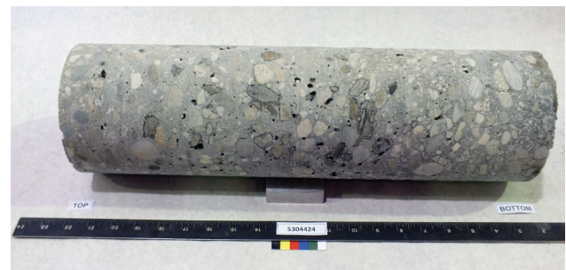
Figure 4 Photograph of air dried core from Mix 1, showing wet rims around coarse aggregate indicative of ASR.
