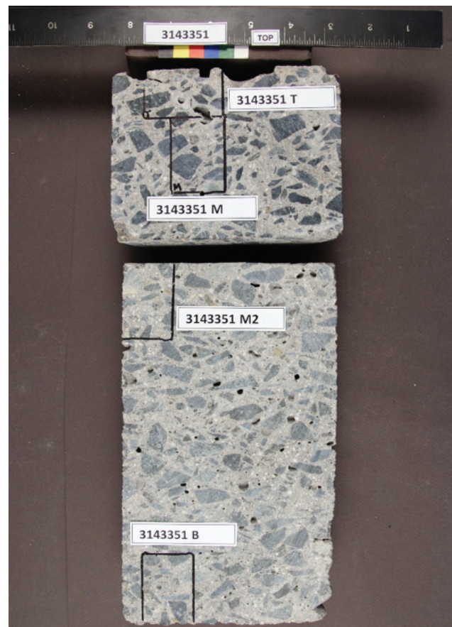
Figure 3 Photograph of cross-sectioned core showing locations of thin section preparation outlined in black
