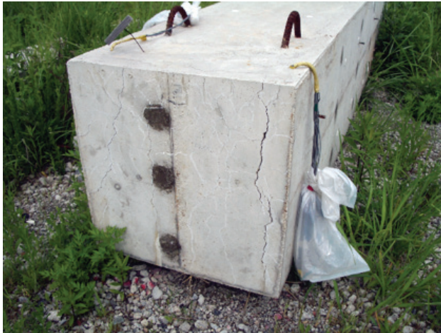
Figure 3 Exposed specimen (at the age of 1.5 years)
