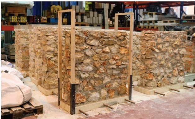
Figure 1 Construction of the masonry specimens at LERM, IST
