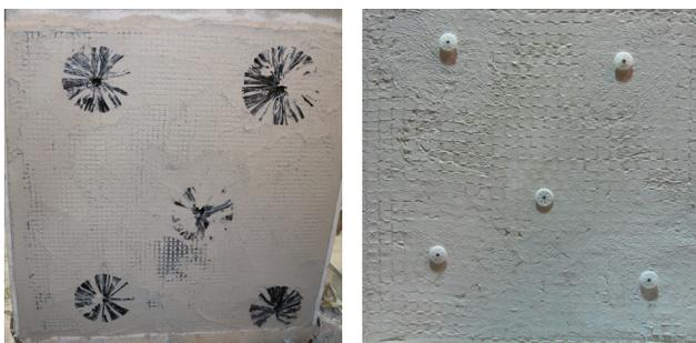
Figure 2 Application of carbon- (left) and glass- (right) FRCM systems on specimens
