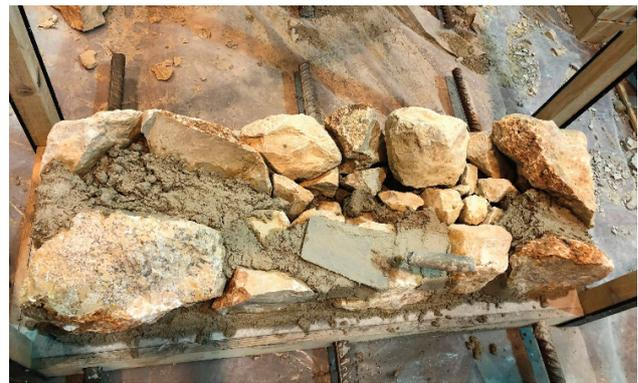
mechanically fixed to the wall, concrete beam, and/or concrete footing, since in many real cases this is not possible to perform (either due to stone edges, or even the impossibility of removing the pavement stones). Connectors are approximately spaced  $50 \text{ cm}$  from the nearest connector, giving a total of 5 connectors per wall. It is worth noting that the holes for connectors were always drilled in the stones.
