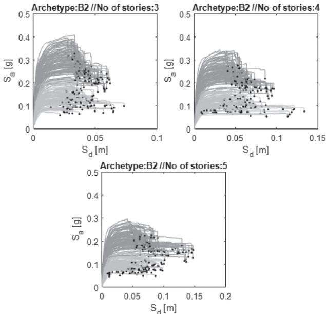
Figure 3 Example of capacity curves for buildings with rigid diaphragm – archetypes B2
