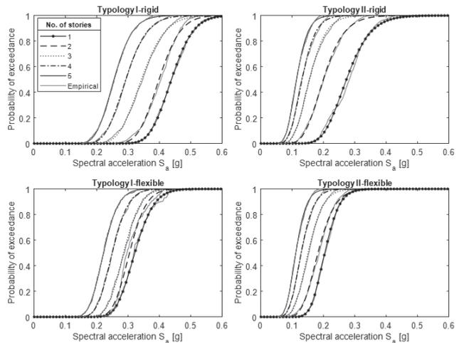
Figure 4 Fragility curves by number of floors, typology and type of floor (rigid and flexible)
