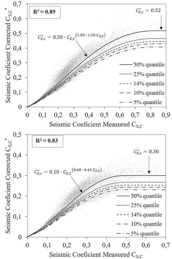
Figure 7 Correction of seismic capacity  $C_{S,C}$  to account nonlinear effects: rigid floors(left) and flexible floors (right)
