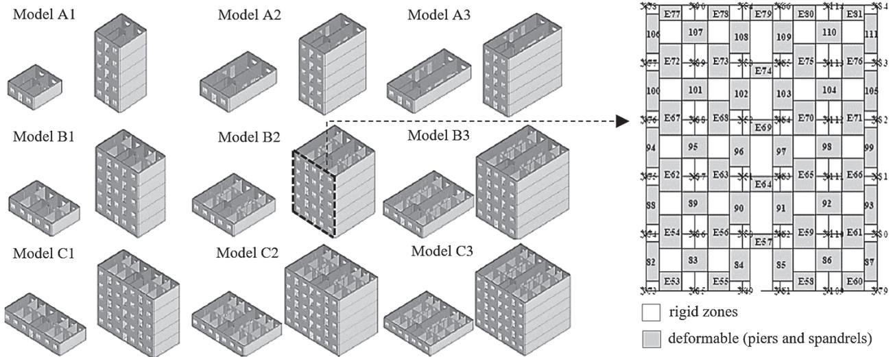
Figure 2 Macroelement models of archetypes (left) and example of equivalent frame model for the facade wall (right)
