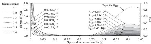
Figure 5 Example of mean annual frequency for a three stories high building, seismic zones 1 and ground type A
