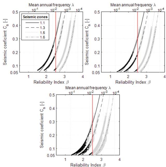
Figure 6 Relation between seismic coefficient and reliability index for offshore scenario (seismic zone 1.1, 1.3, 1.5 and 1.6) and ground type A: buildings with rigid (3, 4 and 5 floors)
