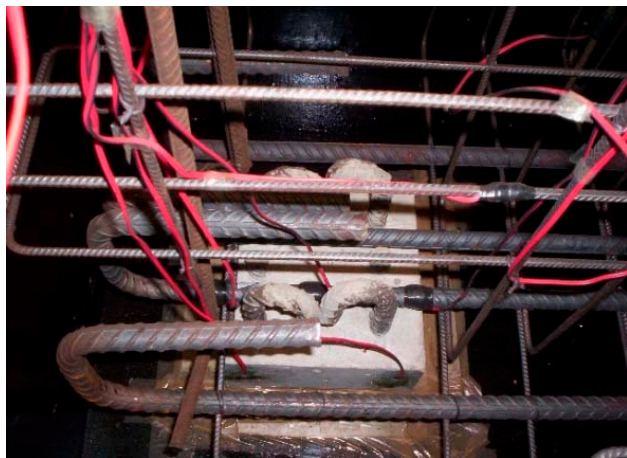
Figure 10 Strain-gages installed the pile head
